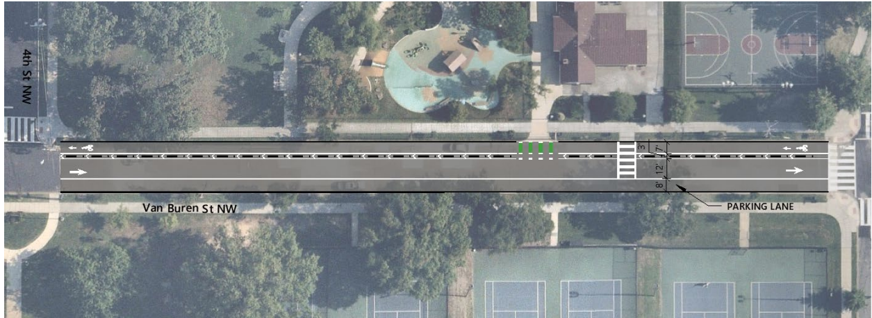
Figure 76. 7-ft Contraflow Bike Lane (6C.8)
