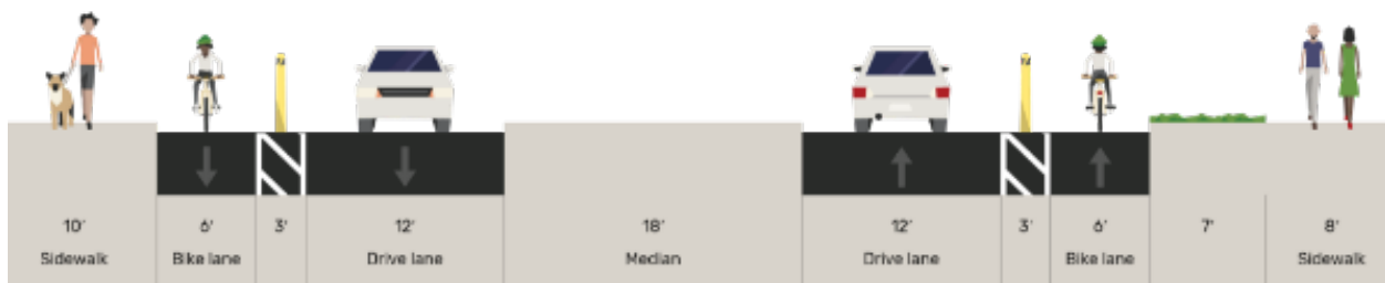
Figure 6. Piney Branch Cross Section - Eastbound
