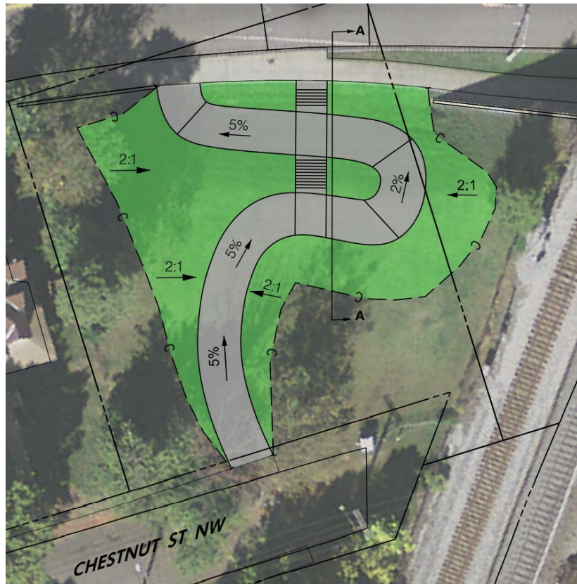
Figure 68. 10-foot Multi-use Curvilinear Path, Staircase and 5,500 SF Green Space (5% slope, max) (2G)
