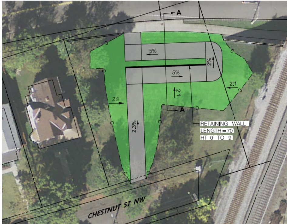
Figure 50. 10-foot Multi-use Switchback Ramp with Retaining Wall and 7,300 SF Green Space (5% slope, max.) (2C)
