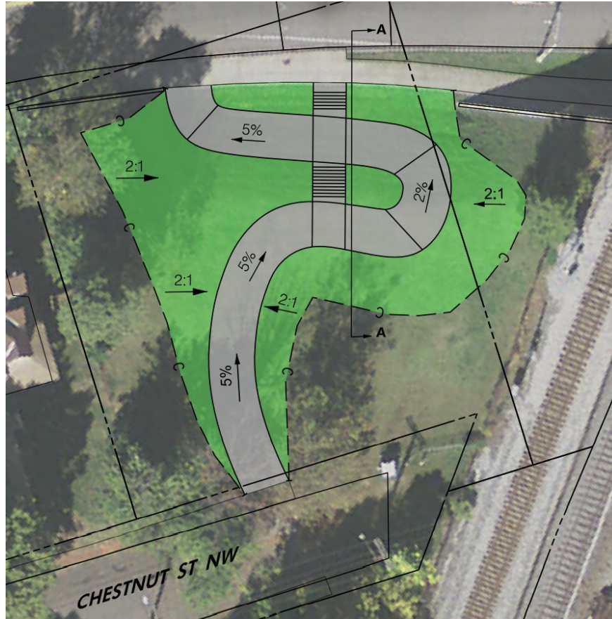
Figure 48. 10-ft Multi-use Curvilinear Path, Staircase and 5,500 SF Green Space (5% slope, max.) (2G)
