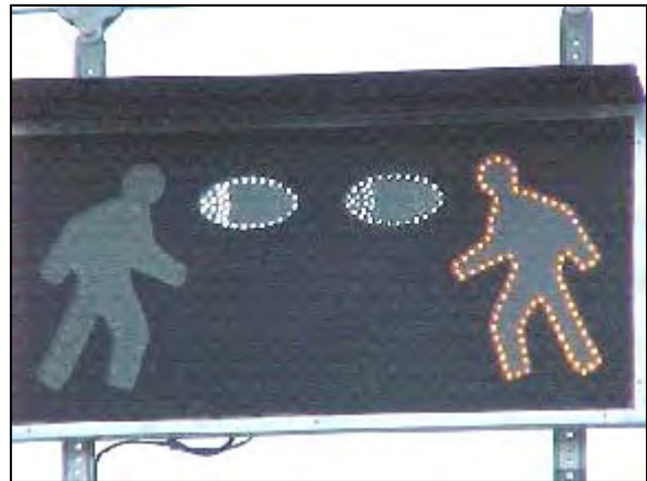
Illuminated eyes look back and forth at 1 cycle/second; the illuminated pedestrian icon (right, left or both) indicates the direction(s) from which pedestrians are approaching.]
